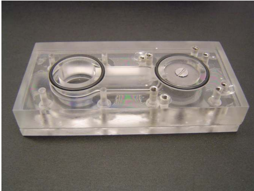
Figure A.9: Anodization chamber used for the production of all of the enriched oxygen targets from the current work.
