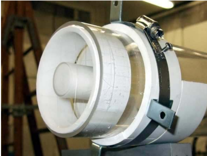
Figure 5.4: The ^{26}\text{MgO} sample suspended in the sample holder. The sample holder consists of a ring with fishing line to suspend the sample. This reduces the amount of material available for Compton scattering, which would produce background in the detectors.
