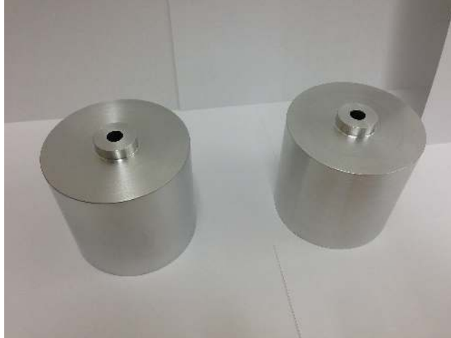
Figure 3.6: Two identical aluminum liners were machined by the UNC Department of Physics and Astronomy machine shop. These liners are 2 mm thick and simplify the separate ceramic bucket and aperture components into one cost-effective and easy-to-machine insert. The natural aluminum oxide layer that forms on the cup is a superb dielectric and maintains the plasma ionization efficiency during operation [93].
