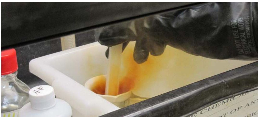
Figure 4.2: All tantalum backings were etched in an acid bath of 5 parts 95% \text{H}_2\text{SO}_4 , 2 parts 70% \text{HNO}_3 , and 2 parts 50% \text{HF} . Etching was performed in a teflon beaker under a fume hood. The necessary safety precautions were taken while etching backings and handling acids.
